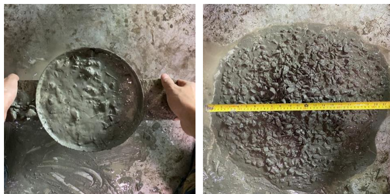
Gambar 3. 2 Slump-flow Test (a), pengukuran diameter (b)
