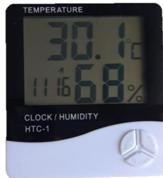
Gambar 6. Alat termometer *hygrometer*.
