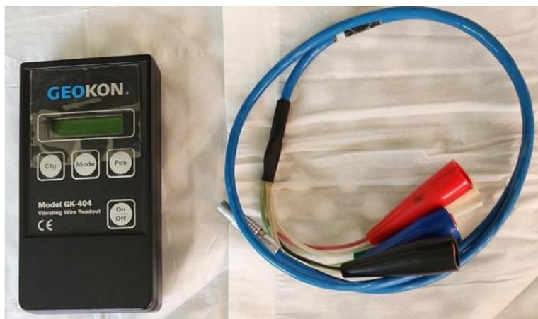
Gambar 5. Alat *vibrating wire readout*.
