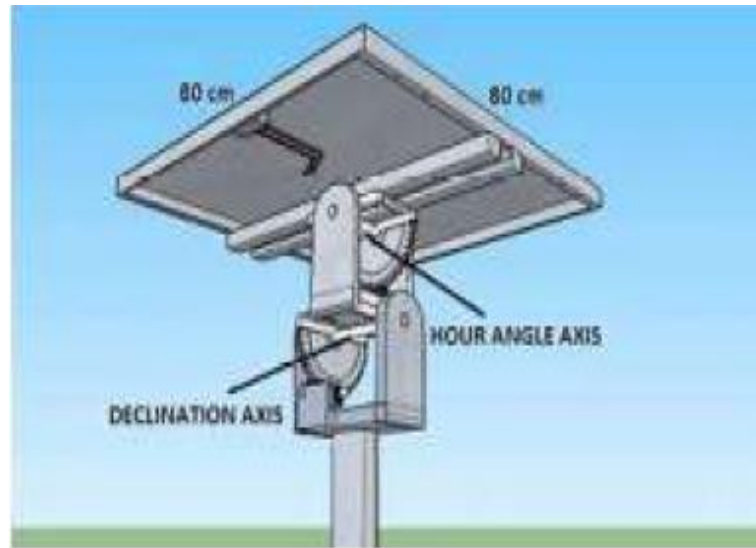
Gambar 2.11 Dual Axis Solar Tracker (Cornelyus, 2021)
