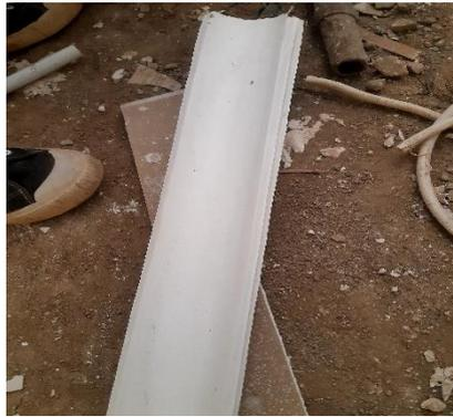
**Gambar 3.23 :** *crown moulding Gypsum*
