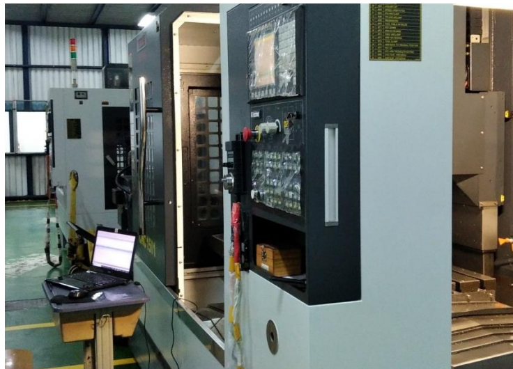
Gambar 3. 4 Mesin CNC Milling 3 axis Merk Feeler VMP40
