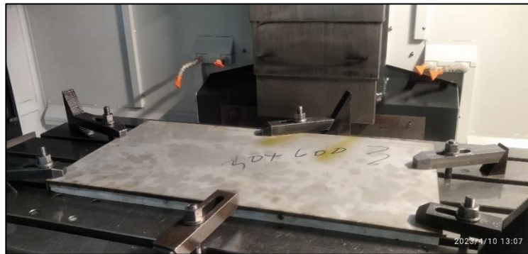
Gambar 3. 9 Setting pencekaman benda kerja
