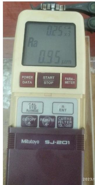
Gambar 3. 6 Surface Tester Merk Mitutoyo SJ201
