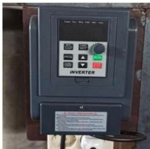
Gambar 3.4 Inverter AC Motor Single Phase
