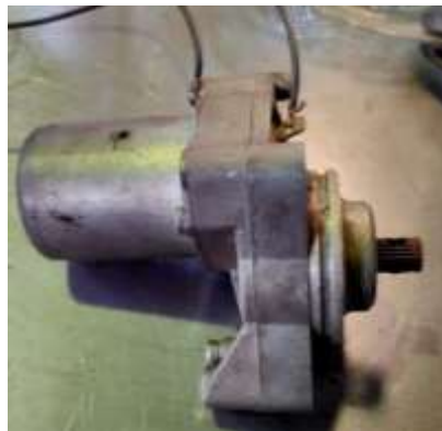
Gambar 3.7 Motor DC Geared
