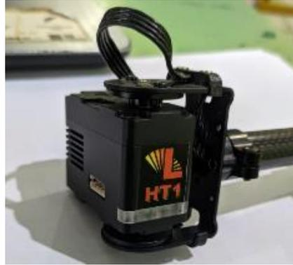
Gambar 2.7 Motor Servo *Lynxmotion*
