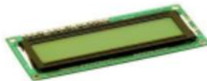
Gambar 17 LCD 2 x 16 Karakter (Rismawan, 2020)
