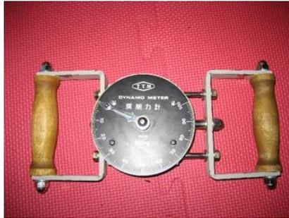
Gambar 10. *Push and Pull Dynamometer*
