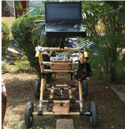
Gambar 3.3. Alat GPR ( Ground Penetrating Radar ).
