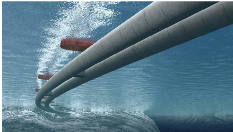
Gambar 1.2 Twin tubes Submerged Floating Tunnel
