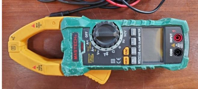
Gambar 3.8 Digital Clamp Meters Voltage Current Resistance Capacitance Tester
