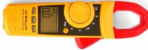
Gambar 2.10 Digital *Clamp-On Multimeter* (Rochim, 2007)
