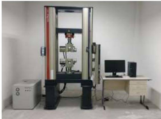
Gambar 14 Mesin Uji Tarik (*Universal Testing Machine*).
