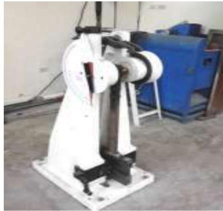
Gambar 15 Mesin Uji Impak (*Impact testing machine*).
