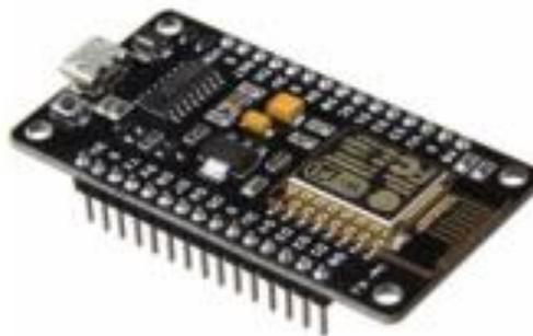
Gambar 2.6 NodeMCU ESP8266
