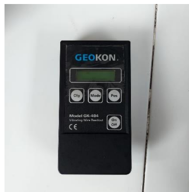
Gambar 3.6. Vibrating wire readout .
