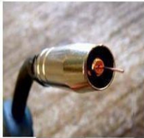
Gambar 5 Nozzle gas pelindung. (Sumber: Widharto, 2007)
