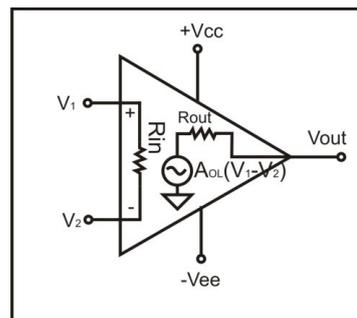
Gambar 2.6. Diagram *schematic* simbol op-amp
