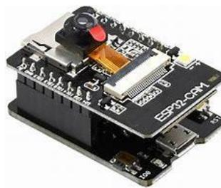
Gambar 1. ESP32-CAM
