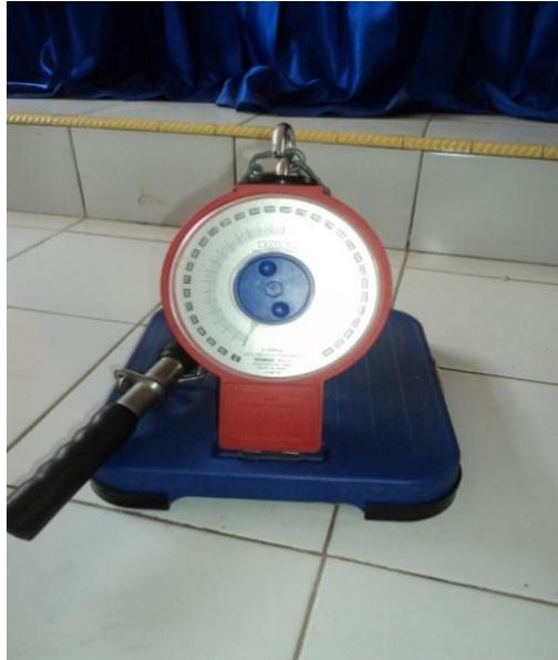
Gambar 5 . Alat *Back and Leg Dynamometer*.
