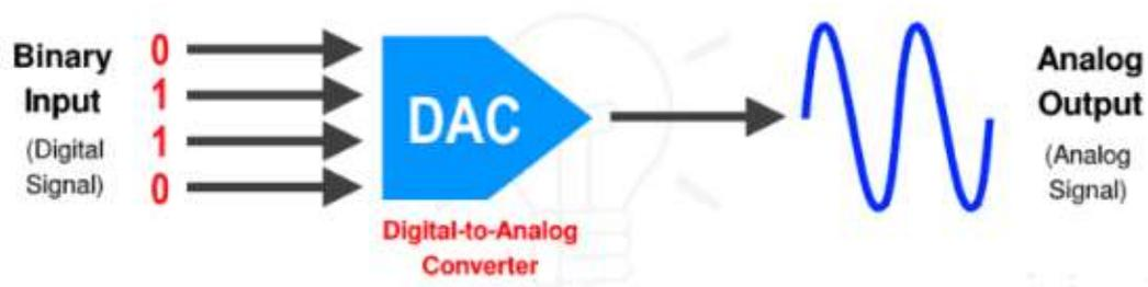
Gambar 2.6 Prinsip Kerja *Digital to Analog Converter*
