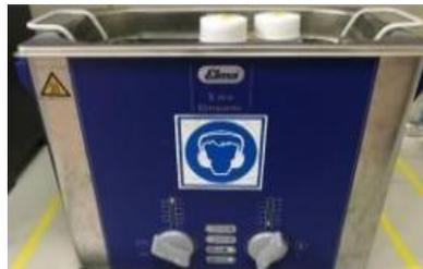
**Gambar 6.** *Ultrasonic water bath* (Aziz *et al.*, 2021).
