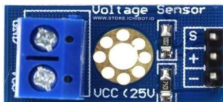
**Gambar 2. 8** Sensor Tegangan DC
