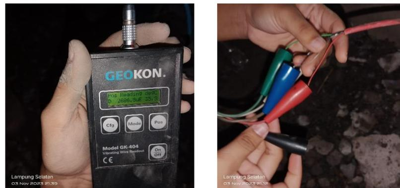
Gambar 3.3. Alat *vibrating wire readout*.
