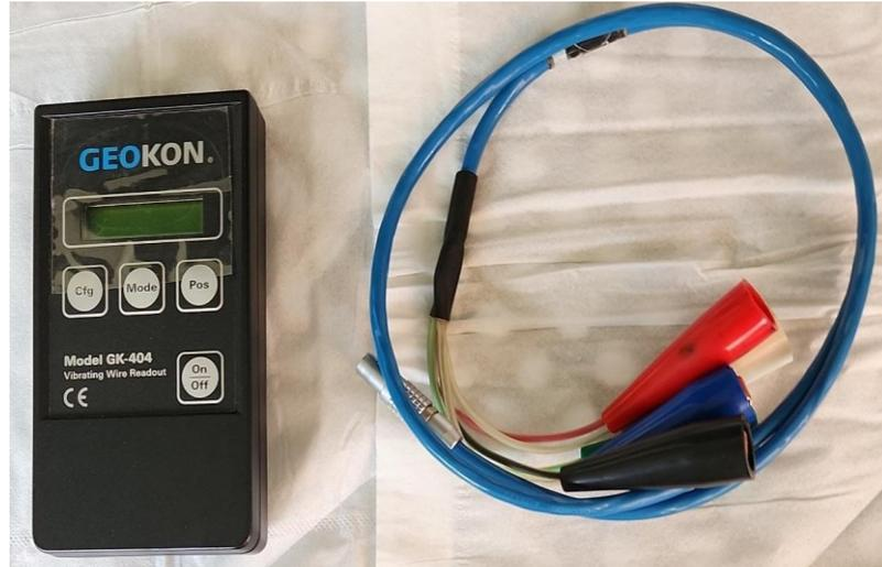
Gambar 4. *Vibrating wire readout.*
