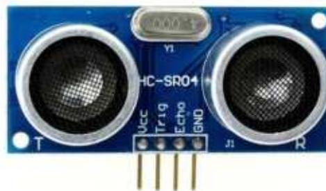
**Gambar 2.6** Sensor Ultrasonik
