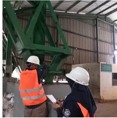
Gambar 23. Pengujian Ultrasonic Thickness Gauge . (Sumber: Survey Penelitian , 2023)
