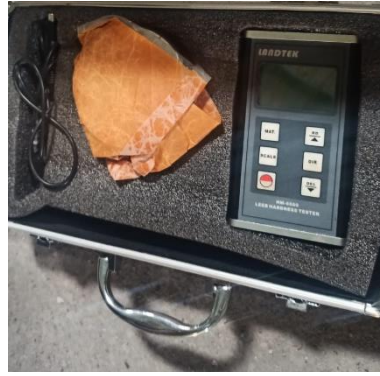
Gambar 19. Alat Hardness Test HM-6580. (Sumber: Survey Penelitian , 2023)
