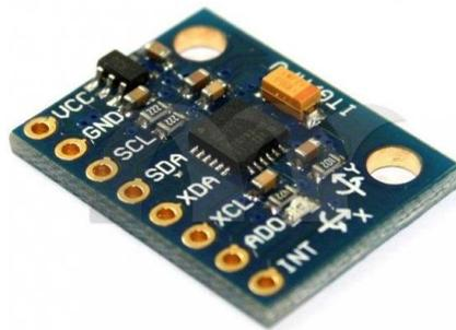
Gambar 2.3 Accelerometer MPU 6050
