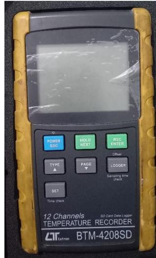
Gambar 3.4 12 Channel Temperatur Recorder Datalogger
