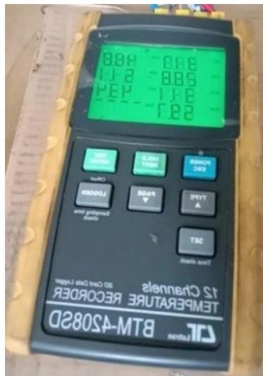
Gambar 3.2 12 channel temperature recorder datalogger.
