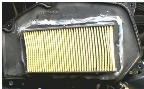
Gambar 5. Filter Udara Kertas (Mughtar, 2017).
