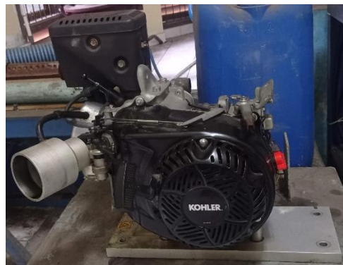
Gambar 9. Mesin Bensin 4-Langkah Kohler
