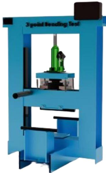
Gambar 3.4. Design Alat Uji *three point bending*
