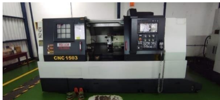
Gambar 21. Mesin bubut CNC FEELER FTC-350XL
