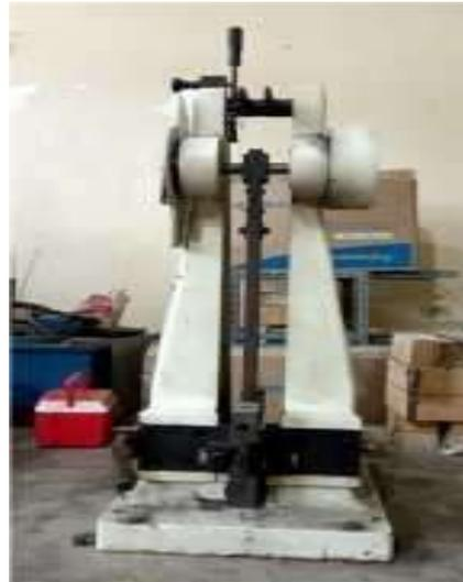
Gambar 22. *Impact Testing Machine*
