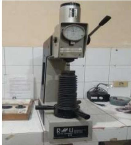
Gambar 17. *Hardness Tester*
