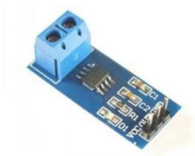
Gambar 2.11 Sensor Arus ACS712
