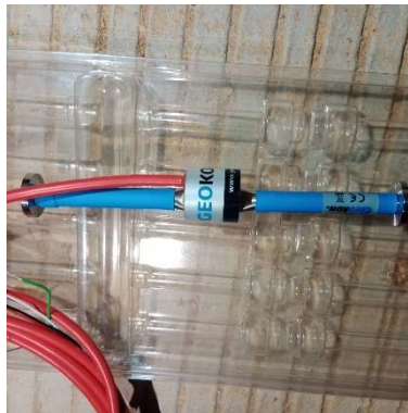
Gambar 9. Embedment Vibrating Wire Strain Gauge (EVWSG) .
