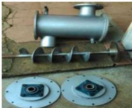
**Gambar 2.11** *Cooling char* tipe screw
