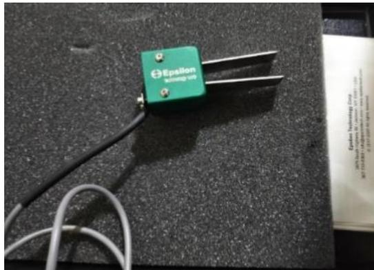
**Gambar 3.5** *Clip on Displacement (COD) Gage*
