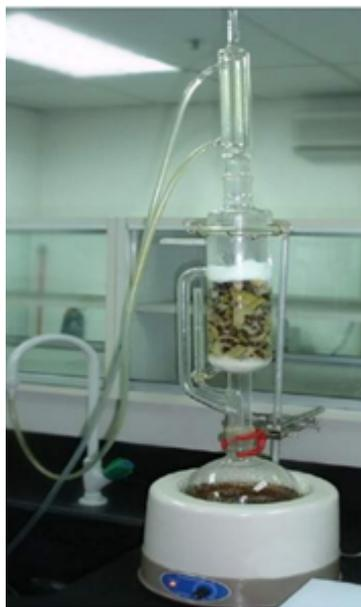
**Gambar 15.** Proses Soxhlet. (Agung, 2017)
