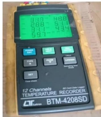
**Gambar 3.2.** 12 Channel Temperature Recorder Data Logger
