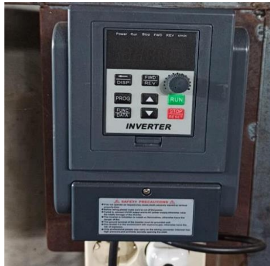
Gambar 3. 5 Inverter AC motor single phase
