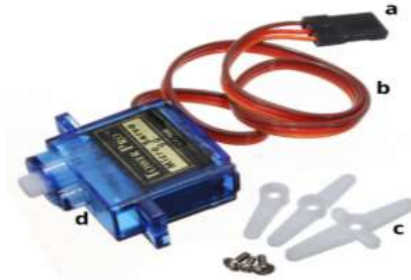
Gambar 2.9 Tampilan motor servo jenis standar (Sujarwata, 2015)
