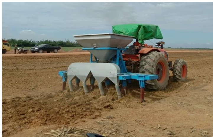
Gambar 7. Alat olah tanah ridger. (Sumber: Tim Penelitian GGP)
