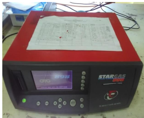
Gambar 3.4. Exhaust Gas Analyzer Stargas 898
