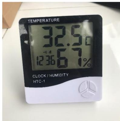
Gambar 3.6 *Thermometer hygrometer*
