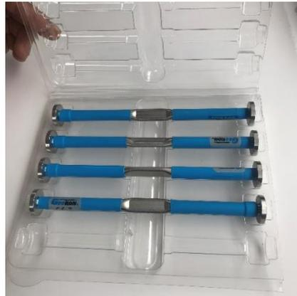
Gambar 3.5 *Vibrating Wire Embedded Strain Gauge*
