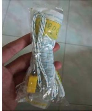
Gambar 3.8 kabel termokopel
