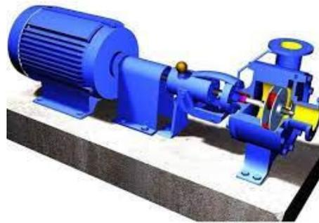
Gambar 2. 5 Pompa sentrifugal
