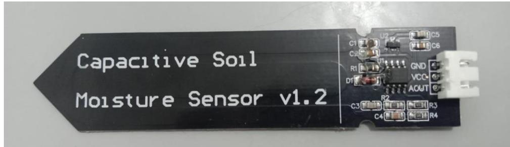
**Gambar 2.1** Sensor Kelembapan Tanah (*Capacitive Soil Moisture Sensor*) (Dokumen Pribadi)
