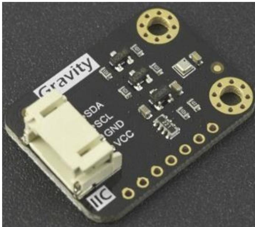
Gambar 2. 8 Sensor Barometrik BMP338.
