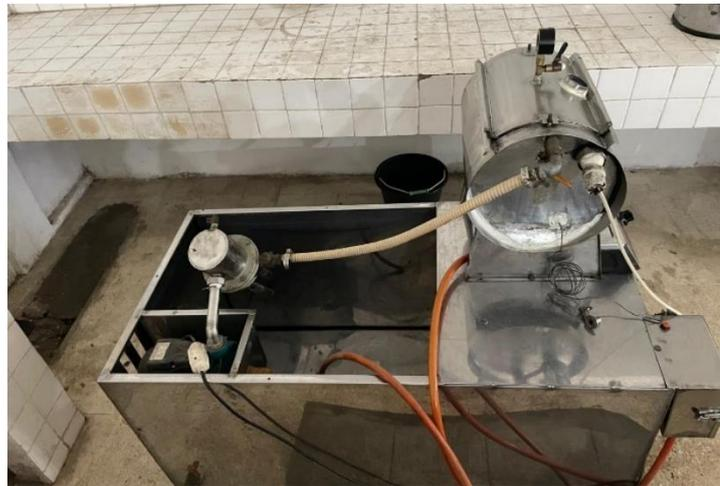
Gambar 2. Mesin *vacuum frying*
