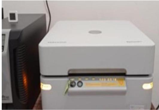
**Gambar 3.** Instrumen XRF Merk Panalytical Epsilon 3 XLE.
