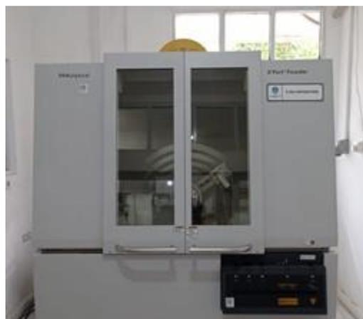
**Gambar 4.** Instrument XRD Merk Panalytical X'Pert 3 Powder.
